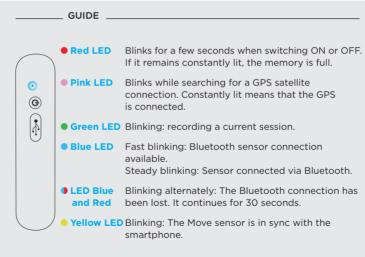
When the sensor is connected to a power source, the LED displays the charging status in green. If the battery level is low, the blinking will become slower. The LED will turn OFF when the battery of your sensor is fully charged.
